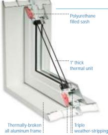
We use a unique exterior trim for superior sealing against air and water infiltration, one which also gives an aesthetic finish to the window frame. Our multiple-air chamber thermal barriers between the exterior and interior frame sections improve energy efficiency and strength.
